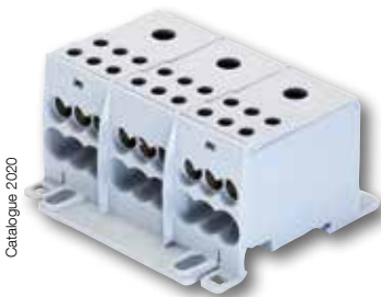
Single-block multi-pole distribution block 175 A 3 P
